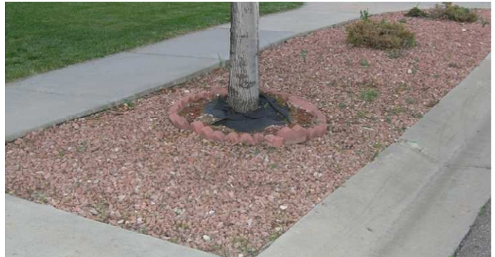
Not this – gravel that is not congruent with any other portions of the streetscape, dead plants, weeds, concrete products, and exposed fabric prevent this parkway from contributing to the street as attractive public space.
