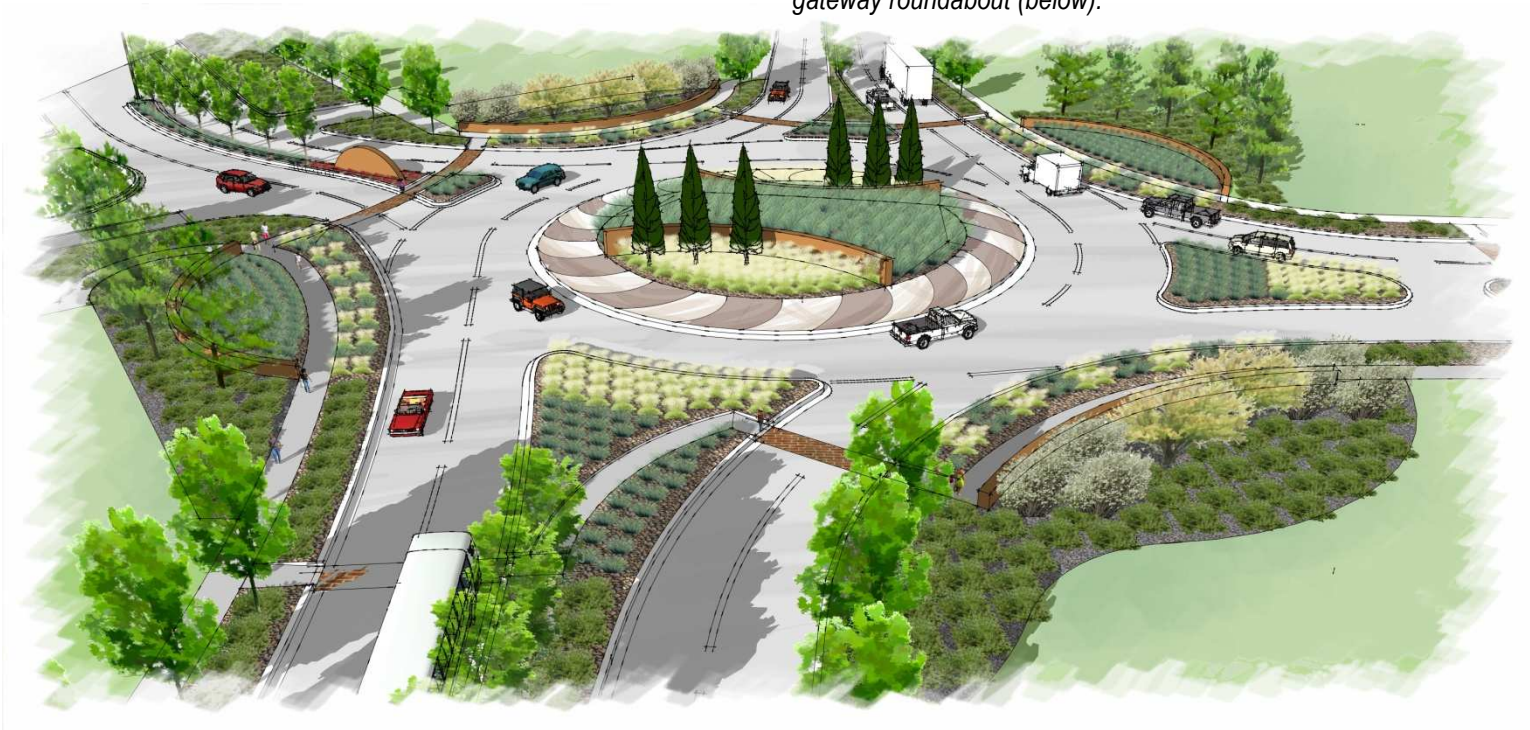
Illustrations of themed plantings, walls, median planters, and specialty paving as examples of special treatments to mark an enhanced gateway signalized intersection (above) and gateway roundabout (below).
