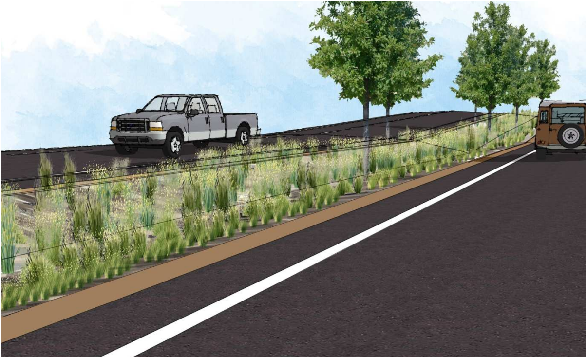
Illustration of LID median concept with street runoff directed to a depressed median with a flush band instead of curb and gutter.
